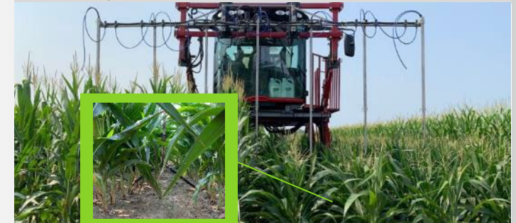
Poseyville, Indiana July 2021 Nitrogen Y-Drops for Precise In-Season Application
